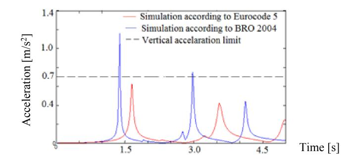
Response due to the force models in ISO 10137 for a group of twenty pedestrians and comparison with the acceleration limit
