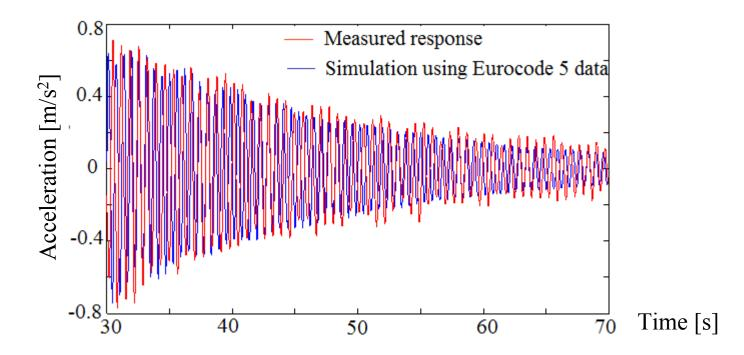
Comparison of measured response and simulations using the simple model according to Eurocode after the group has stopped jumping
