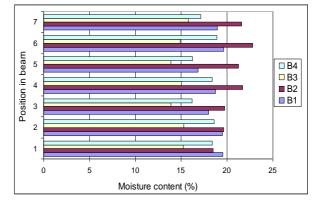
*Fig. 10 Average moisture contents at pins 1-7 in middle of beams, in beam types B1-B4.*
