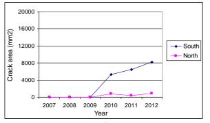
*Fig.* 7 Crack area (mm<sup>2</sup>) in beam type B3, on south and north side, average of five beams
