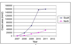
*Fig.* 8 *Crack area* (*mm*<sup>2</sup>) *in beam type B4, on south and north side, average of five beams*
