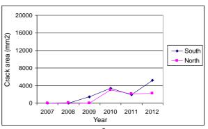
Fig. 6 Crack area  $(mm^2)$  in beam type B2, on south and north side, average of five beams
