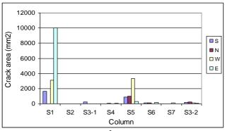
Fig. 11 Crack area  $(mm^2)$  for the different sides south (S), north (N), west (W) and East (E)
