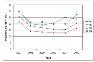
*Fig. 9 Moisture contents in beam types B1-B4, average of all pins 1-7 in middle of beam.*
