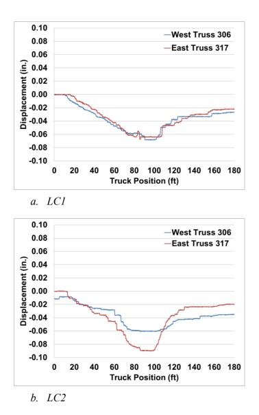
Fig. 5 Global Displacements at Mid Span of the Bridge
