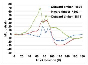
Fig. 7 East Truss Bottom of Bottom Chord, LC3
