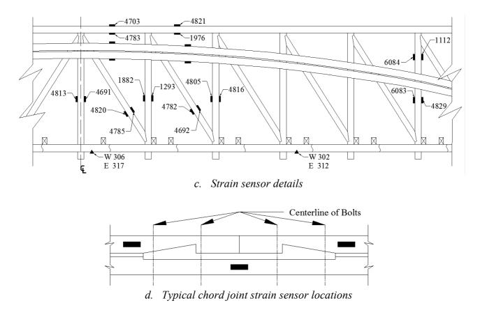
Fig. 2 Strain sensor locations for the Cox Ford Bridge load testing
