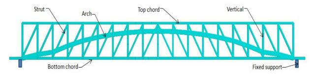
Fig. 8 STAAD model of the Cox Ford Bridge
