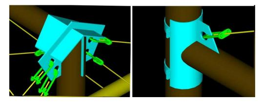
Fig. 4 Design of the footbridge links on the poles.
