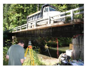
Figure 2. Optical level was also used to collect deflections from calibrated rules suspended from each girder.
