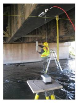
Figure 1. Live load testing data was collected via string potentiometers (deflection) and transducers (strain).
