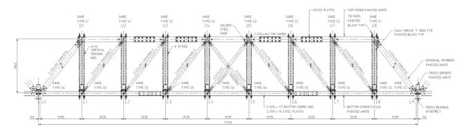
Figure 6 – Side Elevation of the Allen Truss
