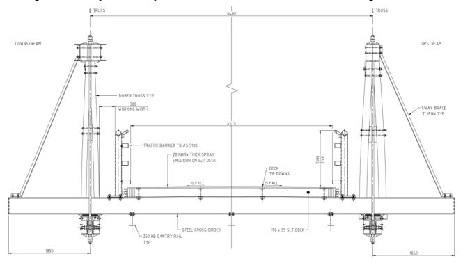
Figure 7 – Typical Cross Section of the new trusses, showing traffic barrier & SLT deck
