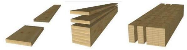
A certain form like a curve is created in step 2 "lamination of layers". The curve is always vertical to the longitudinal axis because the layers only are flexible according to the thickness. Therefore smaller radiuses require thinner lamellas.
