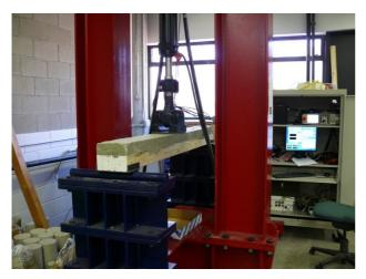
Simply supported specimens were configured with a span of 1524 mm (60 in). Mid-span (threepoint loading) loading was applied using an MTS hydraulic loading and digital data acquisition system. Roller supports were configured at each end to avoid horizontal forces straining the actuator, resulting in a symmetric configuration, see *Fig. 2*. Some of the specimens were subject to static loading while others to cyclic pulsating loading.
