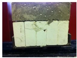
Fig. 5 Typical block-shear failure
