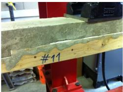
Fig. 6 Typical tension failure
