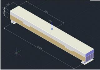
Fig. 1 Specimen configuration [mm]
