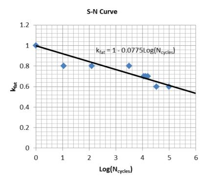
Fig. 4 Mean S-N line approximation
