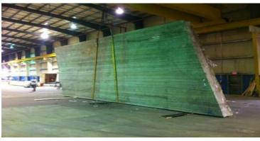
Robust material can be picked up from CL Span And rotated using slings. Picture also shows skew.
