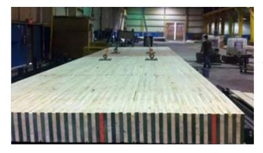
The fiberglass composite slab spans have a manufactured SPF wood core, vertically laminated 495mm deep x 5.018m wide x 11.848m long with a 18 degree skew to be cut after pressing.
