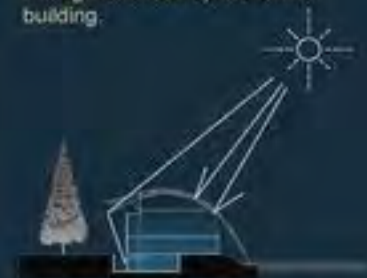
In summer, the closed louvers become heat insulation with two functions – reflecting the sunlight and scattering the interior heat.
