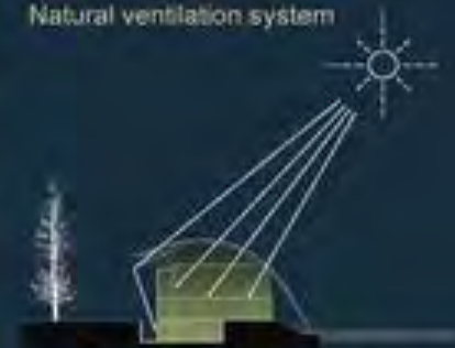
In winter, the adjustable louvers are left open. Sunlight can pass through and heat up the entire building.
