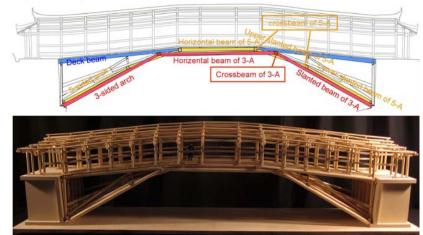
To build a Rainbow bridge we need to build up the whole woven frame at the side as the first step, just as the game shows, and then add in the rest of the beams side by side.
