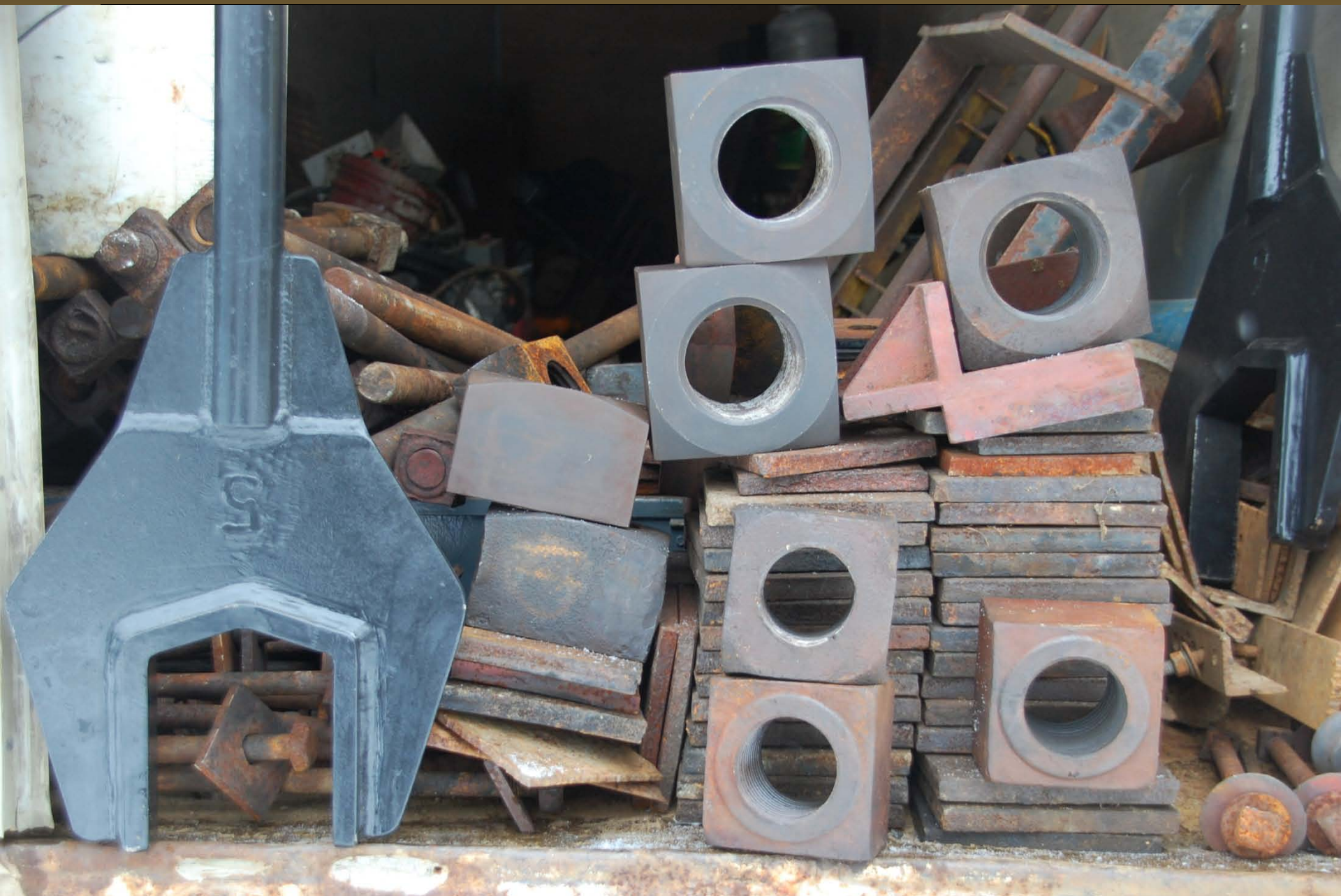
Homemade wrench, 5" for small nuts; three upper nuts are replications
