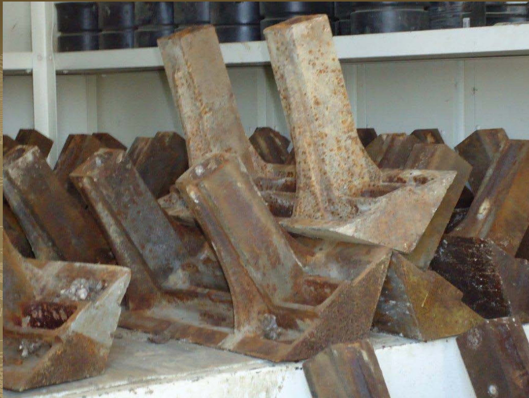
Nodal Castings from Ceylon Covered Bridge in Indiana
