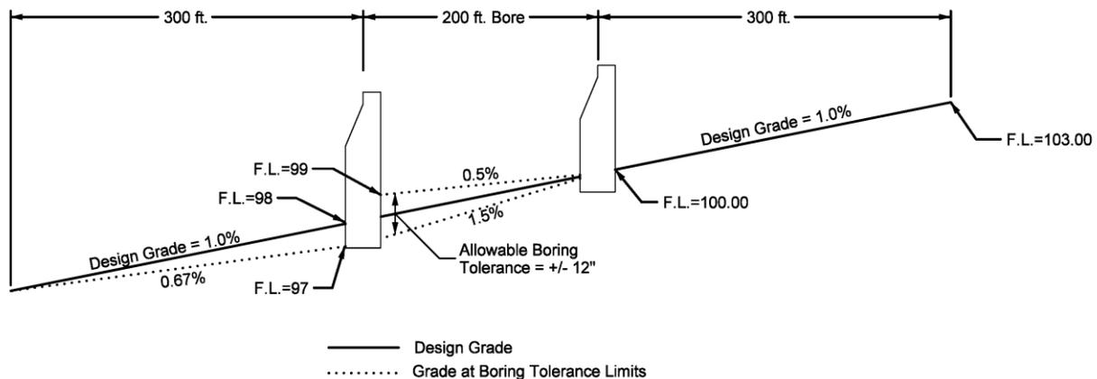
For gravity sewers, which are laid at minimum grades, consideration should be given to providing additional slope through the length of the bore. While this may not always be possible, it helps reduce the potential for backfall in the pipe.
