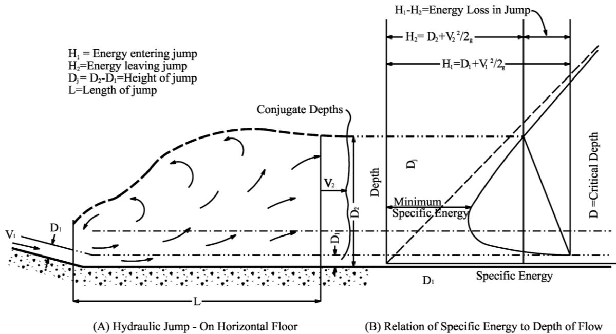
**2. Hydraulic Jump Computations:** The method for calculating the length of the hydraulic jump and the resulting flow depth and velocity downstream of the jump is discussed in detail in FHWA’s Hydraulic Engineering Circular No. 14 (HEC-14), Hydraulic Design of Energy Dissipators for Culverts and Channels. Due to the complex energy calculations required to analyze hydraulic jumps, the use of appropriate hydraulic design software is encouraged.
