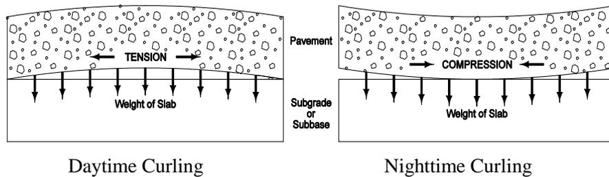
Warping results from a moisture differential from the top to the bottom of the slab. The top of the slab is normally drier than the bottom. The decrease in moisture content causes contraction at the top of the slab, which helps to counteract daytime curling. This contraction causes stresses in the concrete, which can lead to cracking.
