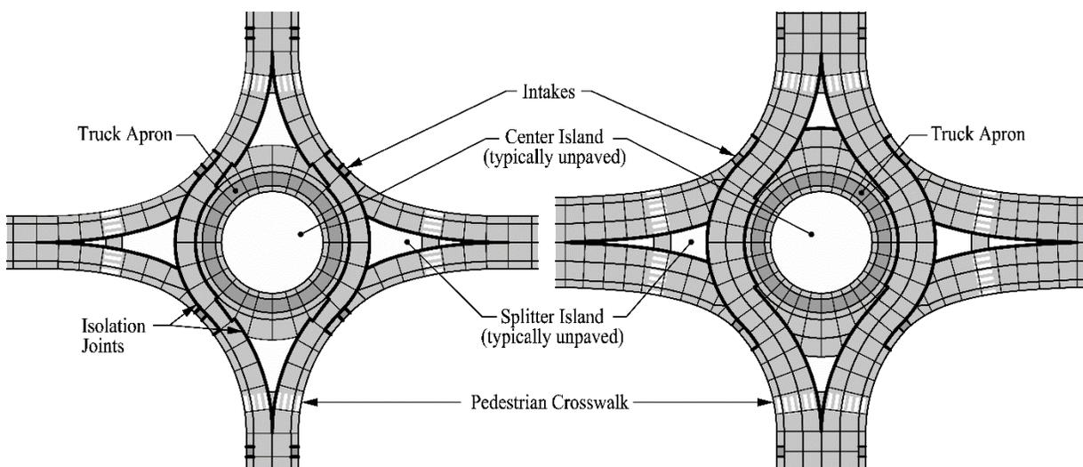
3. **Pinwheel:** This jointing type is sometimes called spiral jointing. It is a combination of the isolation and pave through types. Emphasis is provided for each exiting leg of the roundabout. The jointing for the exit legs is set as for the major pave through legs. The jointing for entering legs is set similarly to the lesser legs of the pave through option. Joints within the circle are set to radiate from the center and the others are perpendicular. See Figure 5G-6.03.
