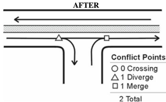
**Figure 5L-3.06:** Two Lane Roadway with Raised Median (left turn ingress allowed into driveway)
