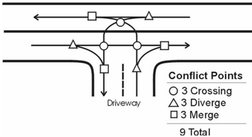
Figure 5L-3.03: Two Lane Undivided Roadway (Closely Spaced Entrances)
