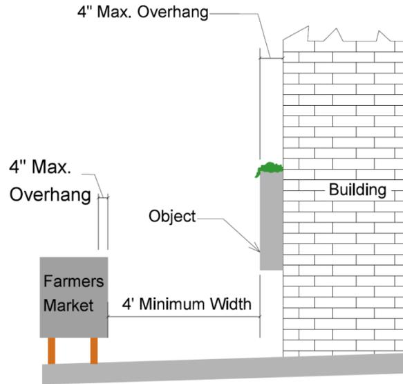
3. **Objects Mounted Between Posts:** Where an object is mounted between posts or pylons and the clear distance between the posts or pylons is greater than 12 inches, the lowest edge of the object shall be between 0 and 27 inches or 80 inches or more above the ground (see Figure 12A-3.05). For objects mounted on posts closer than 12 inches, follow the requirements for horizontal clearance defined above.
