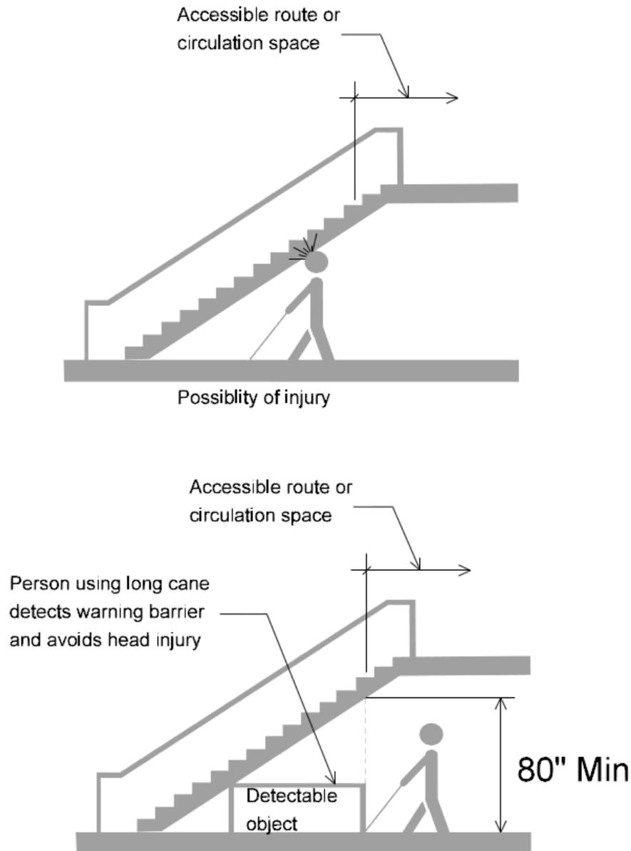
2. **Horizontal Clearance:** Objects mounted at or below 27 inches may extend from a fixed structure into the pedestrian area, provided the remaining sidewalk width complies with Section 12A-2. Objects that extend below 27 inches are easily detectable by most pedestrians.
