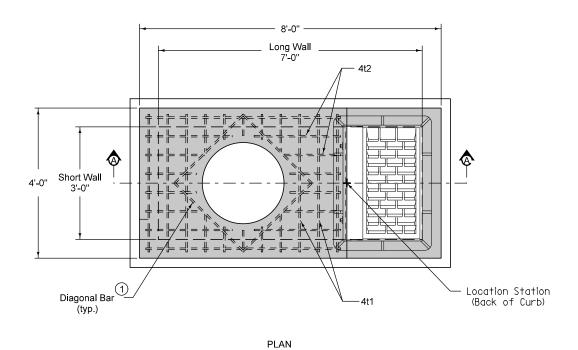
1 Install four #4 diagonal bars at manhole opening and at all pipe openings.
