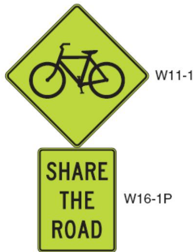
Figure 12B-3.01: Share the Road Sign Assembly
