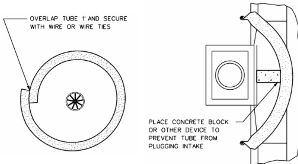
Silt fence, placed around the perimeter of an area intake, can also serve as an inlet protection device. Silt fence used around an intake should be reinforced with 6 by 6 inch welded wire fabric, placed on the inside of the silt fence and securely attached to the posts. Silt fence should not be placed where concentrated flows are expected.
