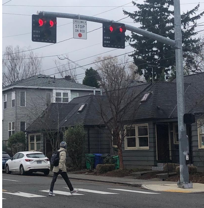
Figure 12A-5.04: Pedestrian Hybrid Beacon
