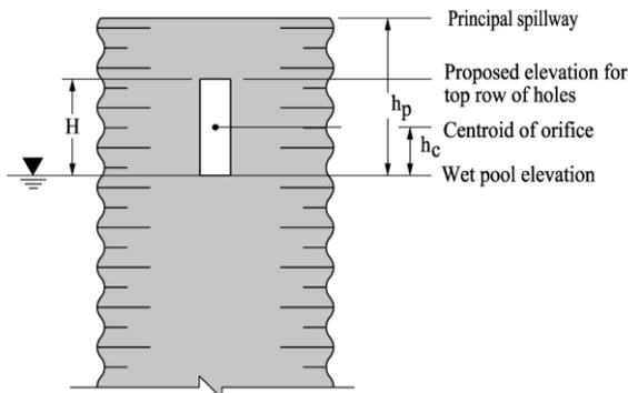
Once the average head is known, the area of the rectangular orifice is sized according to Equation 7E-12.04 to provide the average flow rate for the 6 hour drawdown. Providing evenly spaced perforations that have a combined open area equal to that of the calculated rectangular orifice, will provide the desired discharge rate for a 6 hour drawdown.
