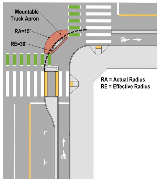
The outside edge of a truck apron (i.e., closest to the travel lane) is constructed using a mountable curb and should be designed so passenger vehicles follow this mountable curbline at the desired speed. Larger vehicles, including SU-30, can traverse the truck apron if desired, but the intersection control vehicle should be used to determine the effective radius.
