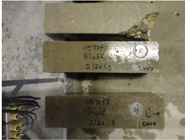
Figure 1. Concrete prism F-T specimens after cracking failure (Bluff City Bartlett Coarse Aggregate)
