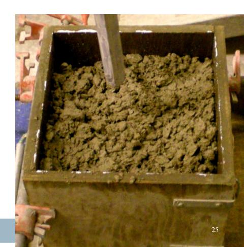
A 1" diameter stinger vibrator is inserted into the center of the box over a three count and then removed over a three count
