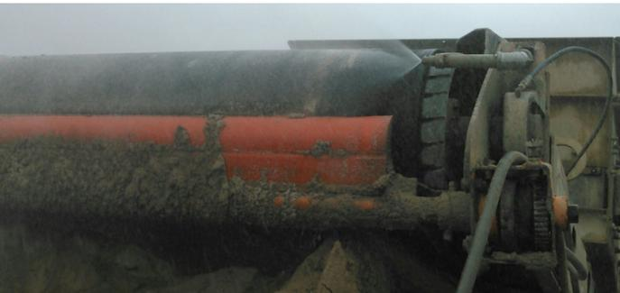
Figure 3. Water spray dust suppression system on concrete crusher (photo courtesy of Duit Construction)
