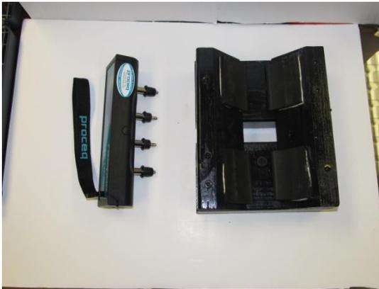
3. Dip the Wenner array probe tips into a pan of water to get the contacts wet.
