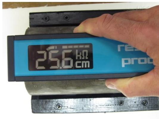
5. Make sure the specimen is saturated surface wet, and place specimen on holder with the 0-degree mark on top.
