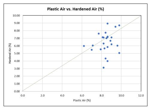
Figure 14: Plastic Air versus Hardened Air Content (%)
