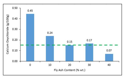
Figure 15: CaOXY formation for different fly ash replacement rates
