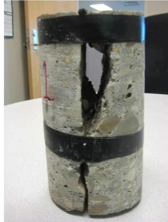
Joint deterioration – Can be caused by backer rod
