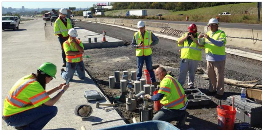
Figure 32: MCL Staff performing the SAM test
