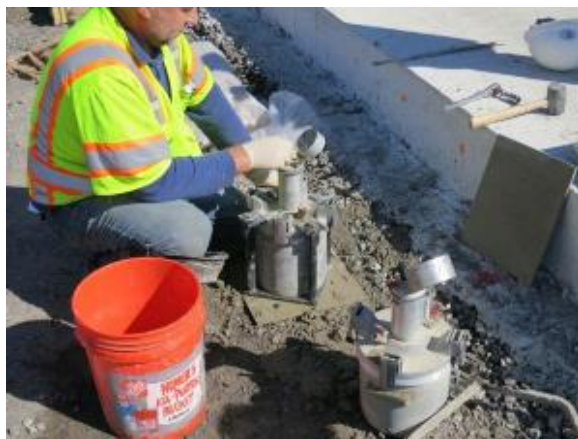
e. Air test (Super-Air Meter [left] and Standard Volumetric Air Meter [right]).
