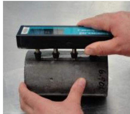
Figure 37: Surface Resistivity Meter in Operation
