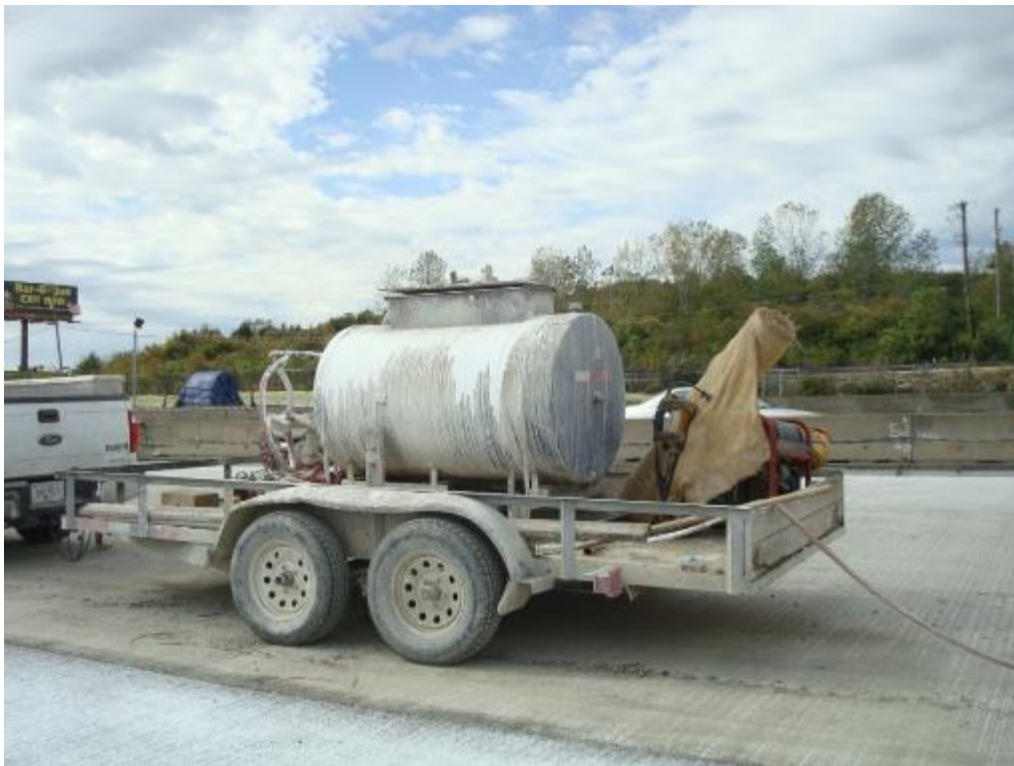
Photo E-52. Cure cart for surface applications.
