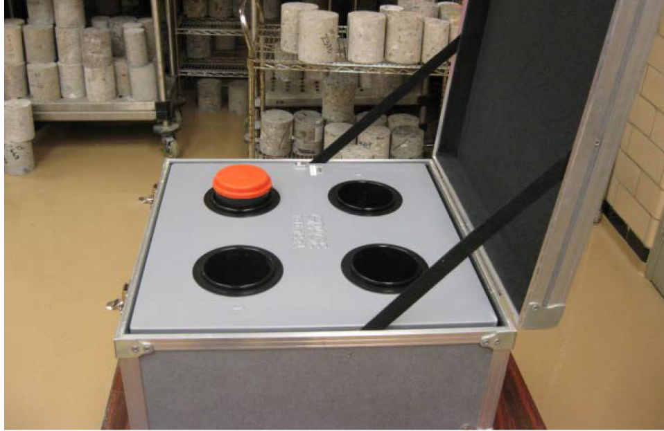
Figure 19. Photo. Semi-Adiabatic calorimeter.
