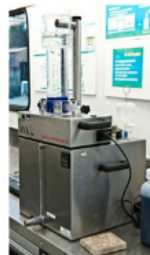
Figure 30: The Air Void Analyzer (AVA)
