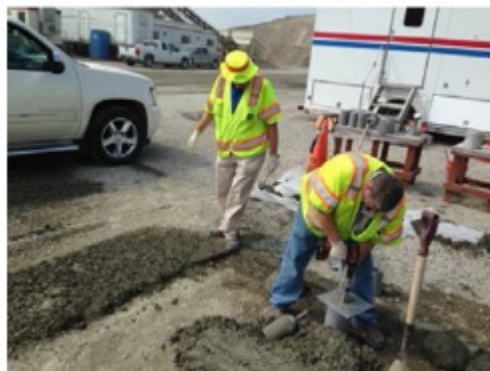
Figure 29: AVA sample being taken from a cylinder
