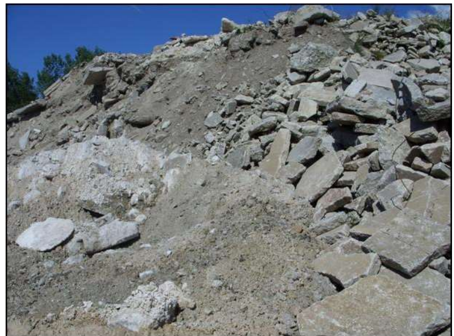
Stockpile of broken concrete with excessive fines
