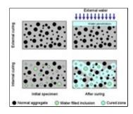
compressive strength, and reduced ion diffusion. It is becoming increasingly clear that internal curing has great potential for the concrete industry to create a longer lasting, more sustainable product.
