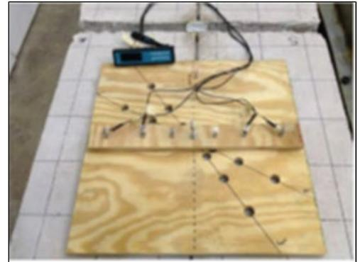
As concrete becomes saturated, its electrical resistivity decreases. Measuring the electrical resistivity between probes placed on either side of a joint was found to be an effective method for determining whether the concrete surrounding the joint was saturated. In addition, measuring the difference in resistivity between probes placed perpendicular to the joint versus probes oriented near the axis of the joint successfully indicated whether the joint contained standing water.
