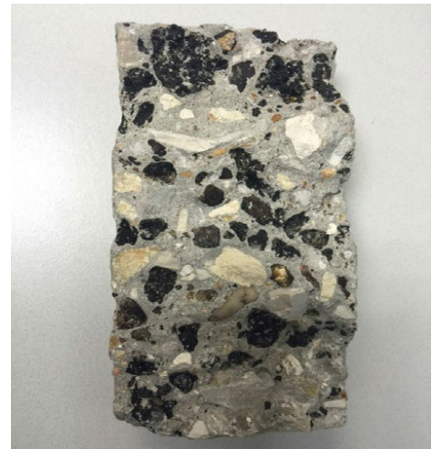
Agglomerated RAP particles in concrete cylinder
