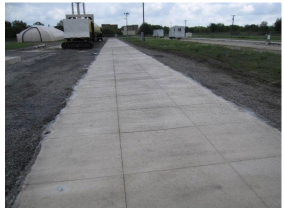
Full-scale thin FRC overlay
