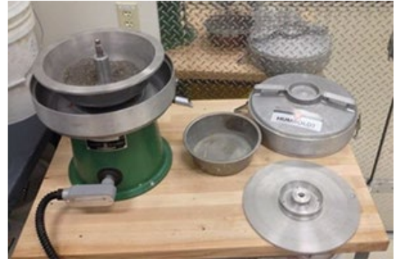
Centrifuge used to determine the moisture properties of lightweight fine aggregate
