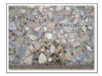
Structural longevity is improved with ICC due to its small reduction in unit weight, elastic modulus, and coefficient of expansion, along with a small increase in strength. When combined, these small improvements amount to a significant impact on slab fatigue damage and slab cracking. Likewise, durability is improved through moisture loss control and improved hydration. ICC shows a reduction in permeability, joint disintegration, and curling.
