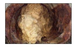
subbase in PCC pavements results in tufa formation, a primary cause of drainage outlet blockage in JPCP.
