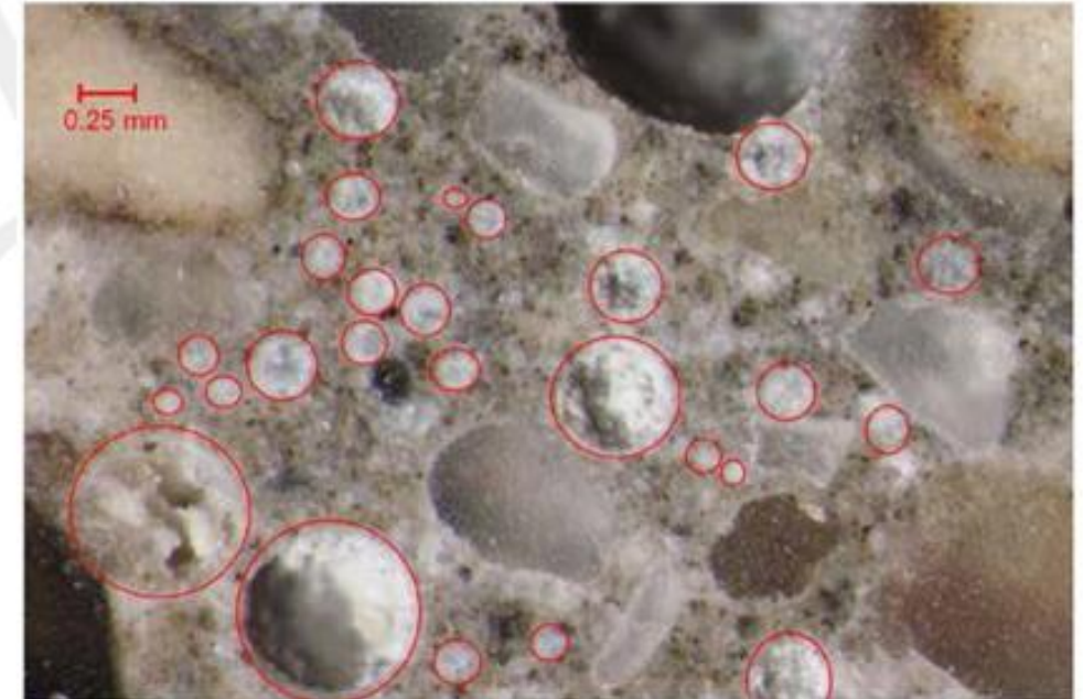
Figure 13b – Air voids Filled with Ettringite
