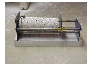
Nine-point core length measuring device
