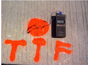
Maturity probe location with hand held thermometer
