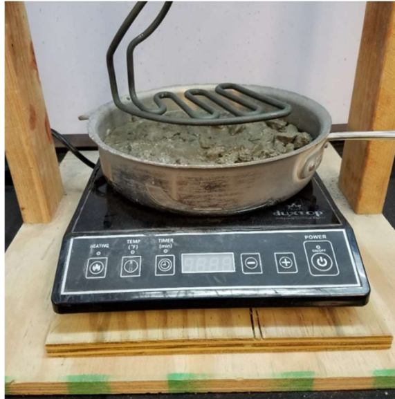
Figure 6. Phoenix test apparatus [Photo provided by Robertson and Ley of Oklahoma State University]
