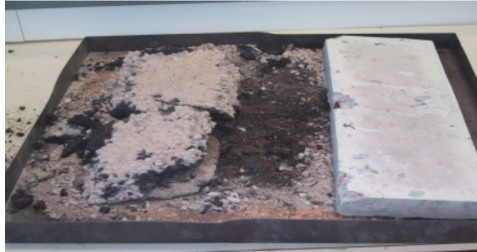
Figure 1 Comparison of specimens of asphalt (left) and concrete (right) after heating to 750°C
