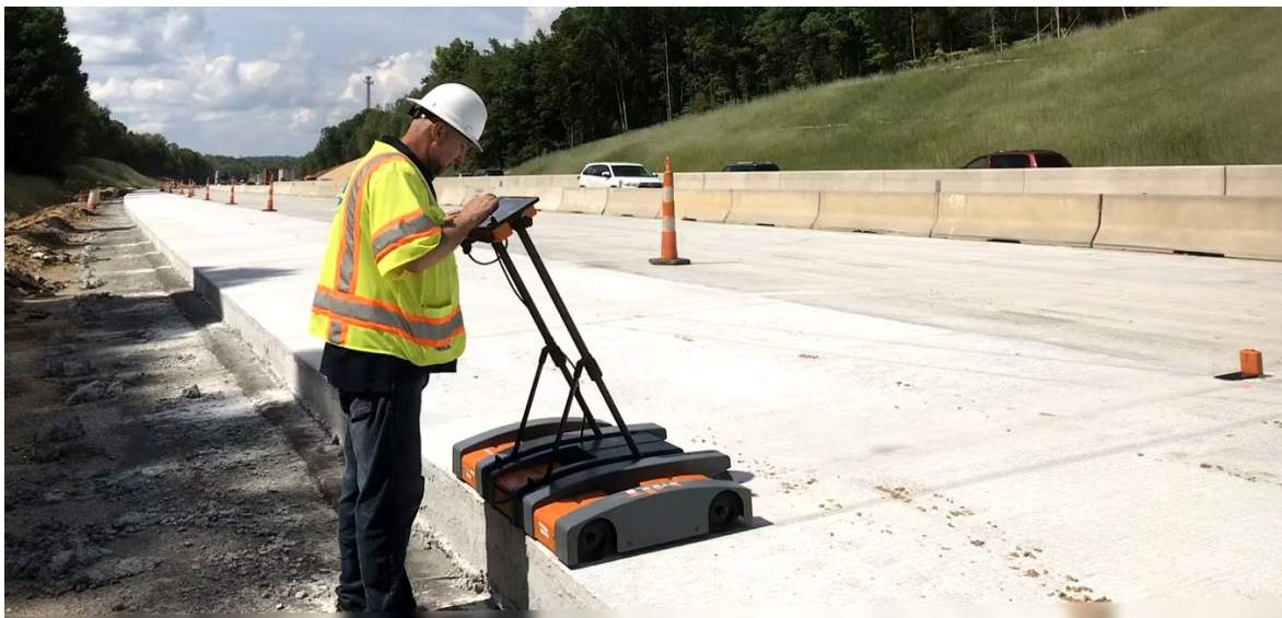
MCTC Personnel using the MIT Dowel Scanner on Shoulder Section
