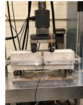
ASTM C1609-12 testing a 6x6x18 in 3 flexural beam
