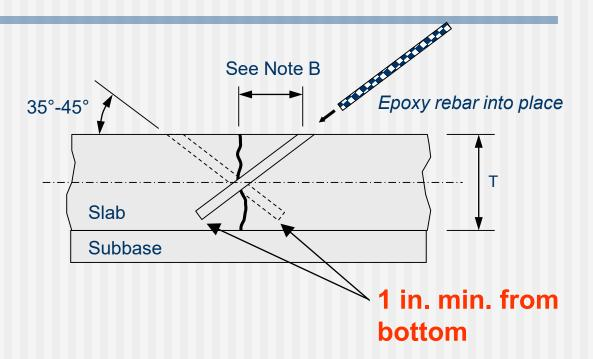
**Note A:** Distance between holes is 24 in. for heavy traffic; 36 in. for light traffic **Note B:** Determine distance from longitudinal crack to hole based on slab thickness T and drill angle. Slabs less than 12 inches thick require a 35° insertion angle.
