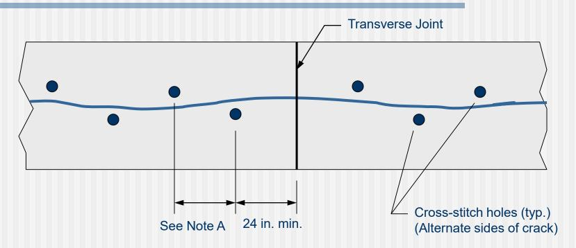
**Note A:** Distance between holes is 24 in. for heavy traffic; 36 in. for light traffic **Note B:** Determine distance from longitudinal crack to hole based on slab thickness T and drill angle. Slabs less than 12 inches thick require a 35° insertion angle.
