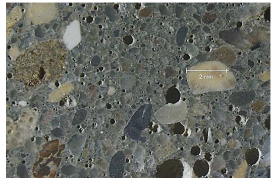
Magnification: 15x Description: Hardened air void system.
