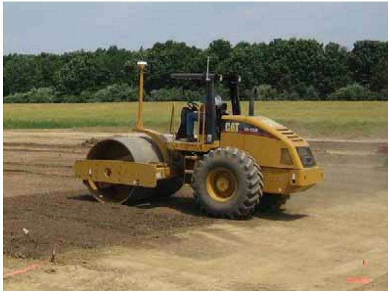
Figure 63. Caterpillar CS-533 vibratory smooth drum roller
