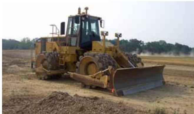
Figure 2. Caterpillar self-propelled non-vibratory 825G roller
