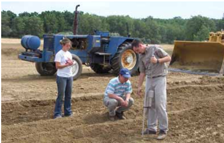
Figure 7. Soil strength measurement using dynamic cone penetrometer
