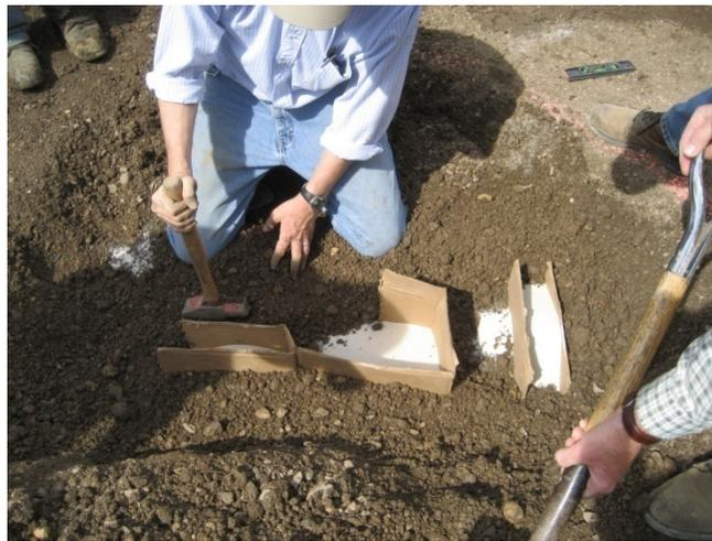
**Figure 16. Placement of sand (~ 2 in) around the EPCs**
