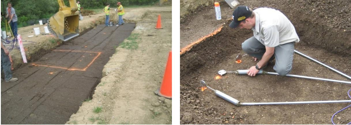
**Figure 13. Excavation to install EPC's (left) and installation of EPC's in orthogonal directions**
