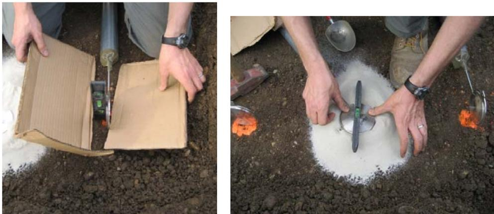
**Figure 14. Leveling of EPC's and placement of thin layer of silica sand below EPC's**
