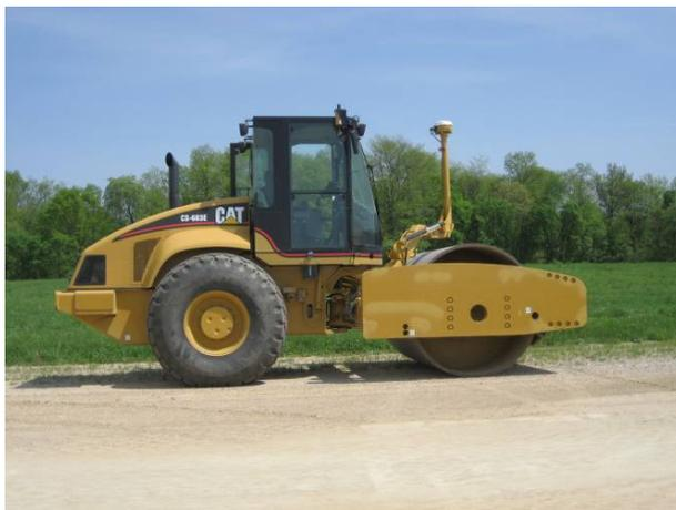
**Figure 18. Caterpillar CS683 smooth drum vibratory roller**
