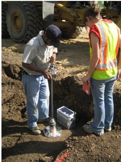
**Figure 48. Process of excavation to the top of each underlying lift to perform LWD and NG testing**
