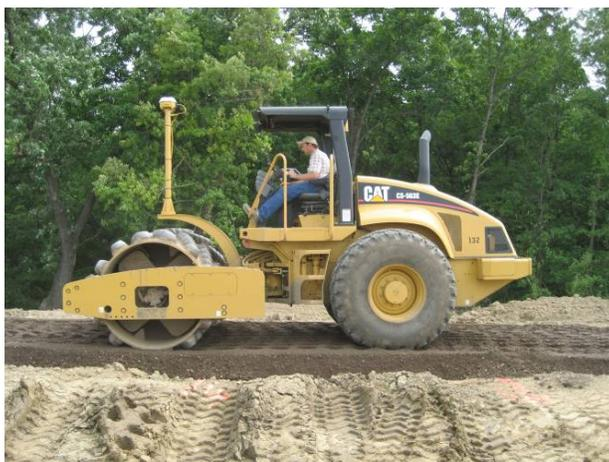
**Figure 19. Caterpillar CS563 padfoot vibratory roller**
