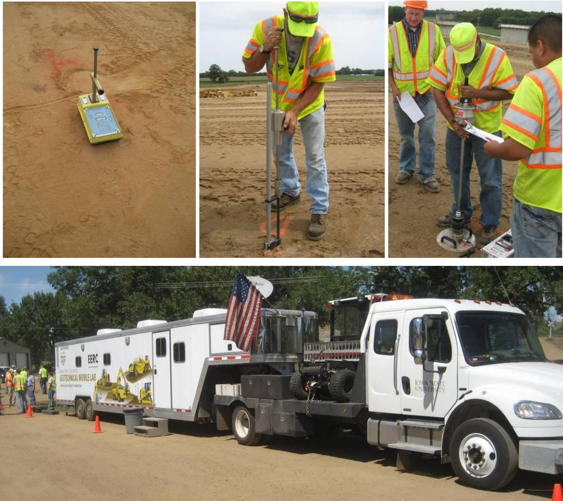
**Figure 3. In-situ testing methods: Humboldt nuclear gauge (top left), dynamic cone penetrometer (top middle), and Zorn light weight deflectometer (top right), and Iowa State University geotechnical mobile laboratory (bottom)**
