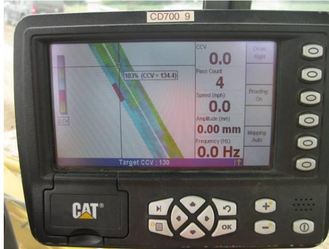
**Figure 2. On board Accugrade display unit showing compaction data in real-time**
