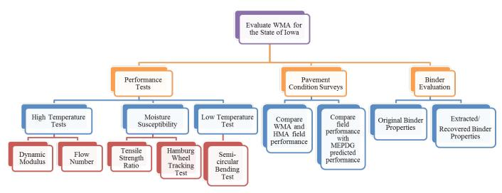
Conceptual diagram of Phase II scope and testing plan
